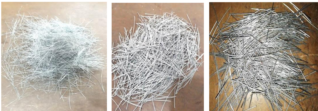
(a) The diameter of 0.50 mm (b) The diameter of 0.70 mm (c) The diameter of 1.00 mm
